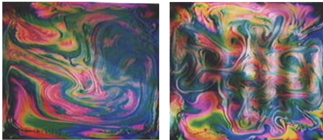
Fig. 1. Onset of vortex flows in a horizontally inhomogeneous liquid film.
